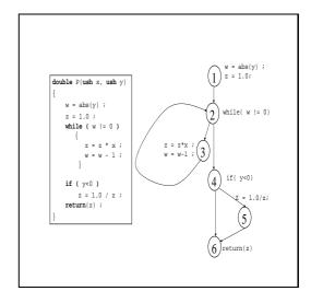
Figure 2: Control flow graph of program power.c
