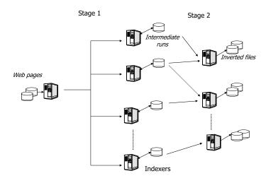
Fig. 11. Text indexing stages
