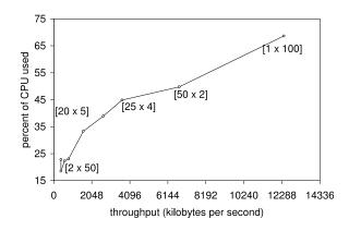
Fig. 7. Throughput of processes versus event loop
