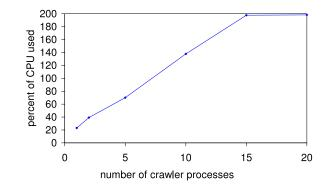
Fig. 8. Crawler CPU usage. Measurements taken when each process crawls 100 sites simultaneously. Point [5, 70] therefore indicates that crawling 500 sites concurrently via 5 processes requires 70% of one CPU.
