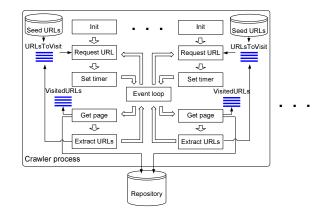
Fig. 5. Crawling multiple sites in a single process
