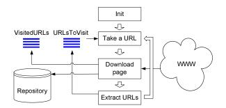
Fig. 2. Conceptual operation of a Web crawler
