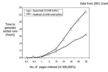
Fig. 12. Performance gain through pipelining
