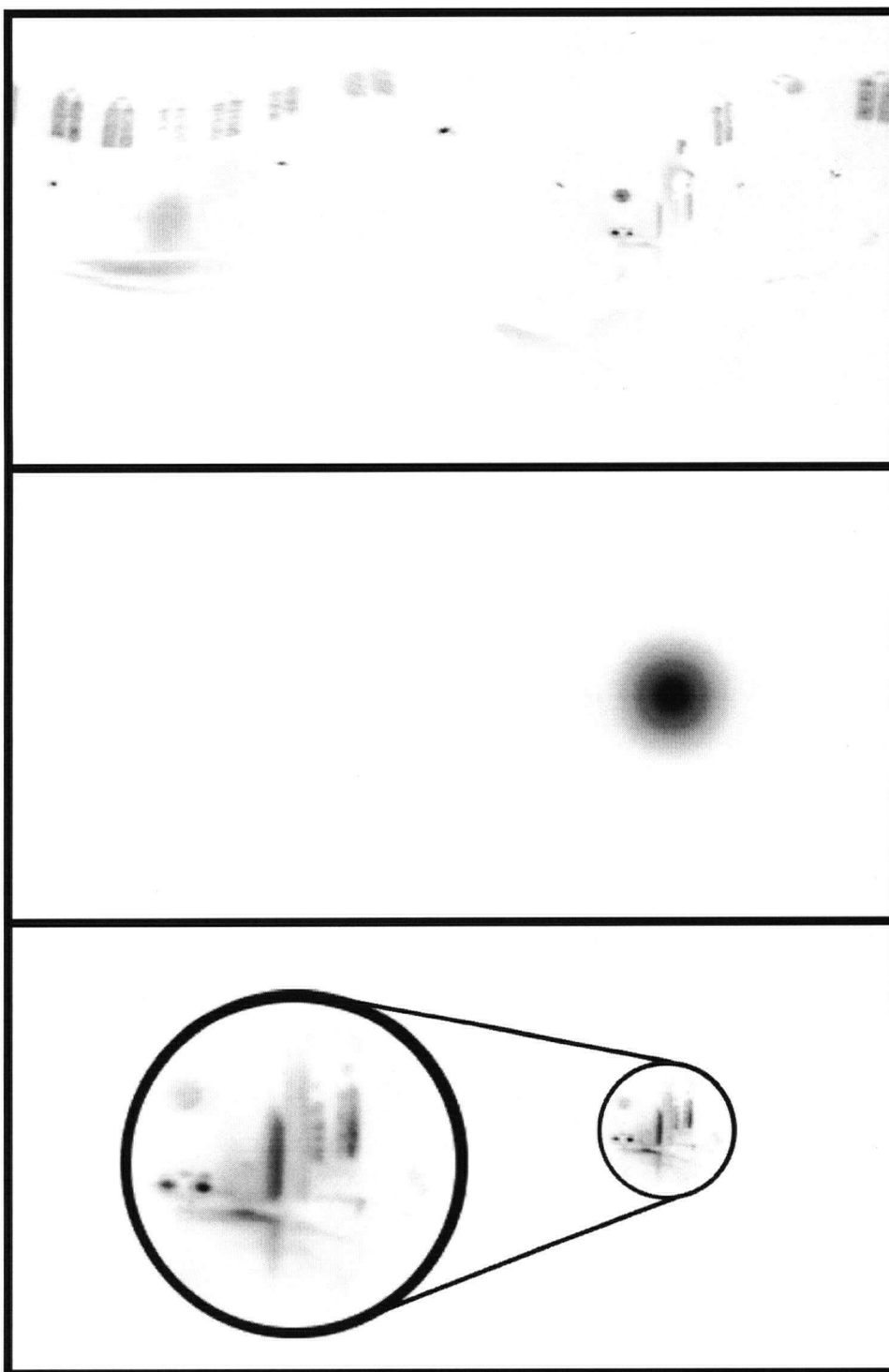
Figure 4.1: From top to bottom: angular plots of the importance function of the Grace Cathedral EM, a specular Phong BRDF of exp 50, and their product.
