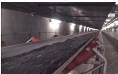
**Figure 4. Underground conveyer belt transporting coal.**
