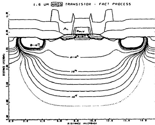
Figure 2 N-channel device cross-section generated by SUPRA.
