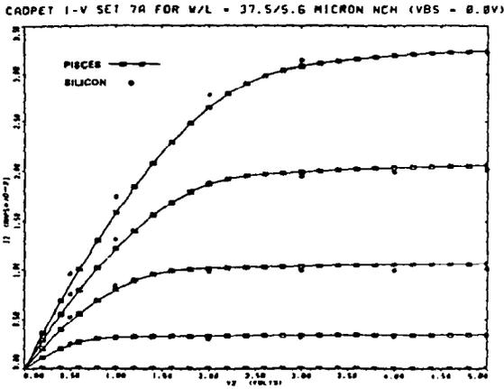
Figure 7 Drain characteristics generated by PISCES for  $W/L = 37.5/5.6$  micron N-channel device, showing comparison with silicon.
