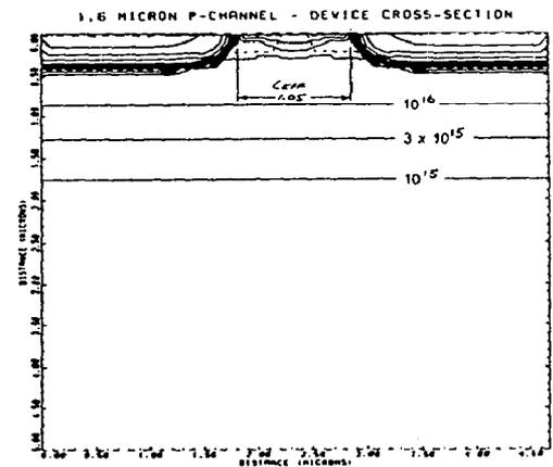
Figure 5 P-channel device cross-section generated by PISCES for minimum 1.6 micron channel length device.  $L_{eff} = 1.05$  micron.
