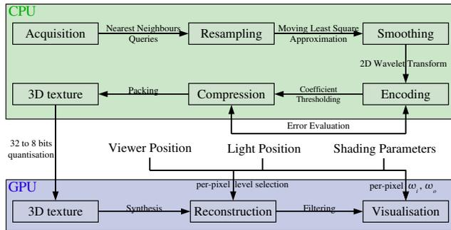
Figure 4: Our BRDF acquisition, encoding and rendering pipeline.
