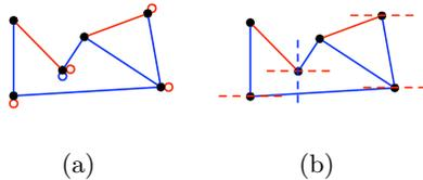
Figure 3: Pinned Laman mechanisms and slider pinning: (a) the combinatorial object; (b) the associated axis-parallel bar-slider framework.
