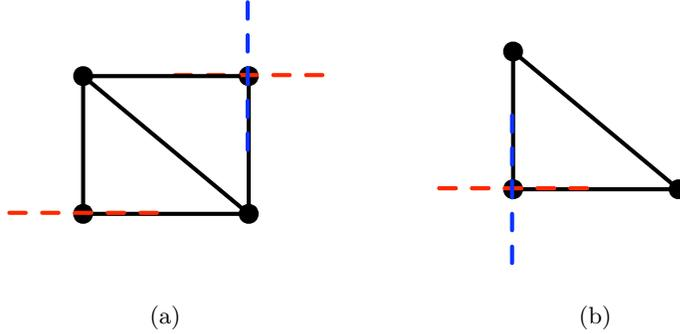
Figure 4: Two embeddings of the same axis-parallel bar-slider framework: (a) generic; (b) non-generic. In (b) one triangle is reflected along the diagonal edge, resulting in coincident vertices and overlapping edges.
