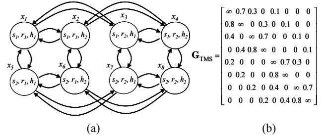
Figure 5. An example of CTMDP model of a TMS (a) and its generator matrix (b).
