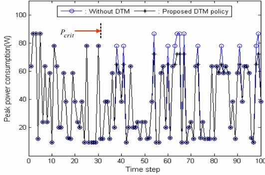
**Figure 7. The effectiveness of the proposed DTM technique.**
