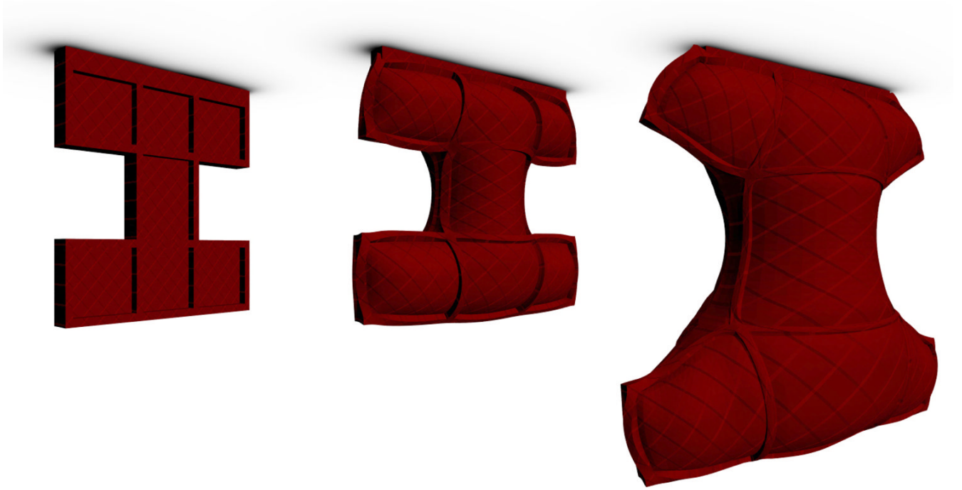
Figure 12. Reanalysis of balloon inflation using cubature optimized from PCA-based simulation data. The dynamic Mooney-Rivlin rubber balloon can be inflated interactively.
