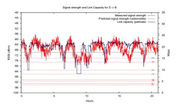
Figure 5: Measured signal strength and link capacity values for the link *S* to *B* over a 24 hour period.
