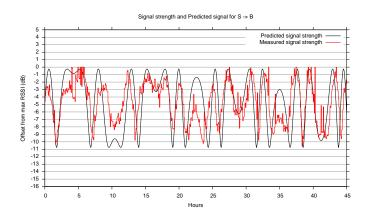
Figure 6: Comparison of measured signal strength values with the values predicted by a simple two-ray reflection model taking into account water level variations over a 45 hour period (almost two days).
