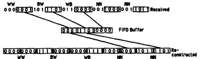
Figure 2. Example of IBC Decoding Procedure, 4-bit Block
