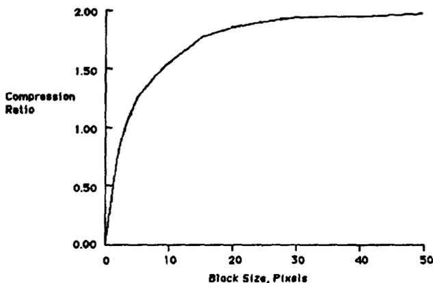
Figure 4. IBC Compression Ratio as a Function of Block Size
