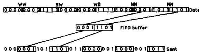
Figure 1. Example of IBC Coding Procedure, 4-bit Block
