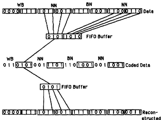
Figure 8. Example of Modified IBC, 4-bit Block, Overflow
