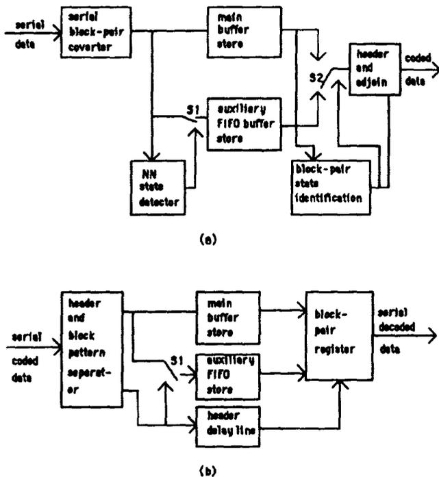
Figure 3. Interleaved Block Coding Scheme
