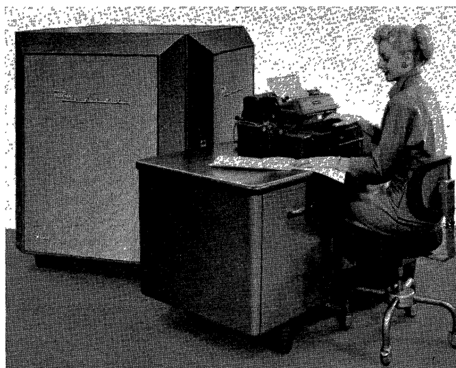
Fig. 7. Standard Marchant MINIAIC computer with Flexowriter input-output. The magnetic tape system supplants the Flexowriter
