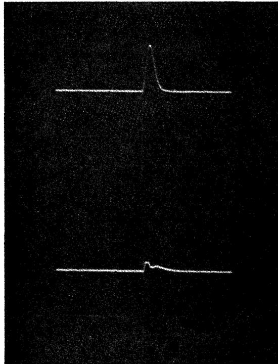
Fig. 12—Signal and noise responses of the relay analog unit. Time scale: 1  $\mu$ sec/cm.
