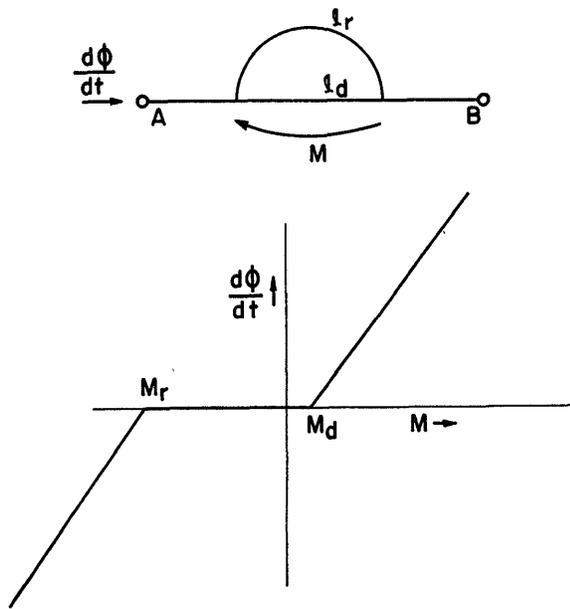
Fig. 13—Magnetic diode terminal characteristics.
