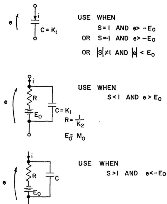
Fig. 2—Equivalent electrical circuits.
