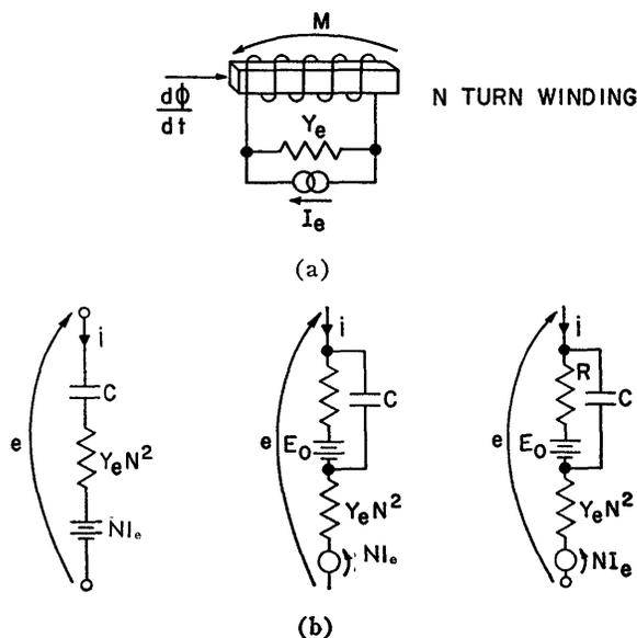
Fig. 3—Modified equivalent circuits for magnetic element coupled to an electrical circuit.
