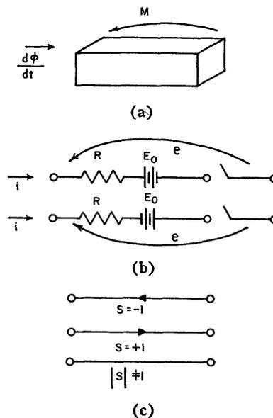
Fig. 4—(a) Elementary unit, (b) simplified equivalent circuits, (c) graphical notation.
