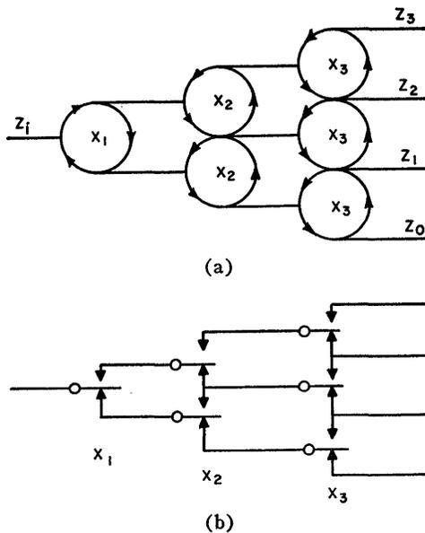
Fig. 11—(a) Relay analog symmetric tree, (b) relay symmetric tree.
