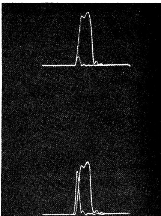
Fig. 7—Flux-steering gate output. Scale: 0.05 v per turn per division (vertical) and 0.2  $\mu$ sec per division (horizontal). Top: unloaded; bottom: loaded.
