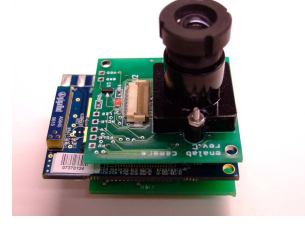
Figure 5: iMote2 with Enalab camera and custom SD card board
