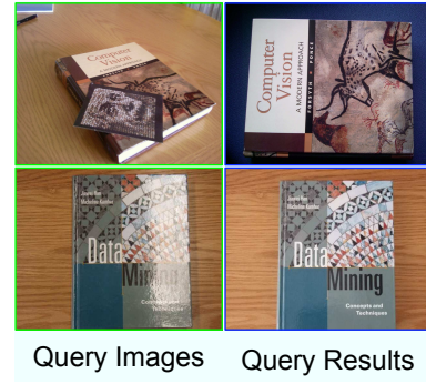
Figure 4: Examples of book cover search results. The first column shows queries and the top results are shown in the second column. The technique is resilient to occlusions and viewpoint change (top left image) and specularities (bottom left image).
