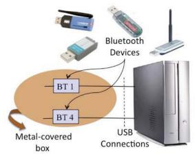
Figure 1. Testbed for the experiments in ideal conditions (without packet retransmissions)
