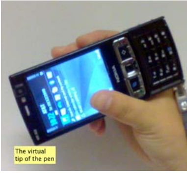
Figure 2: (a) Pretending the phone's corner to be the pen-tip reduces rotation. (b) Raw accelerometer data while drawing a rectangle (note gravity on the Z axis). (c) Accelerometer noise smoothing.
