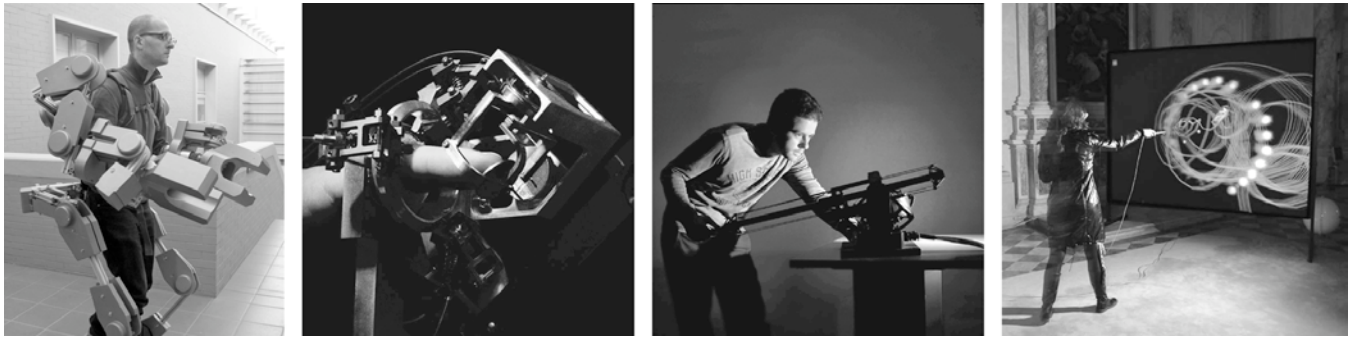
Figure 1. Existing prototypes of perceptual robotic technology. These include, from left to right: the PERCRO Body Extender, an EEG-controlled robotic exoskeleton for manipulating heavy loads in unstructured environments [1]; a novel encountered haptic interface for the finger [3]; the GRAB system, which is easily employed as a general purpose robotic force feedback device [19]; and Passages [11], an enactive interface for artistic expression.
