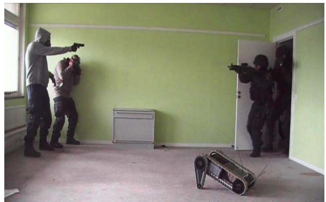
Figure 3. Tactical test of the distraction-siren. From left to right: the officer acting as criminal; the officer acting as hostage; the two SWAT-officers attacking. The hostage taker was instructed to shoot at the police, which he succeeded in despite the siren. The hostage immediately plugged his ears with his fingers. The electronically filtered hearing protection used by the police protected them from the noise.
