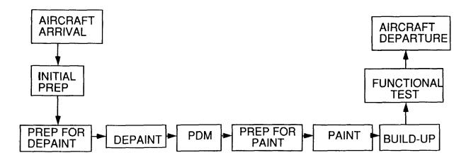
Figure 1: Initial Programmed Depot Maintenance (PDM) Process
