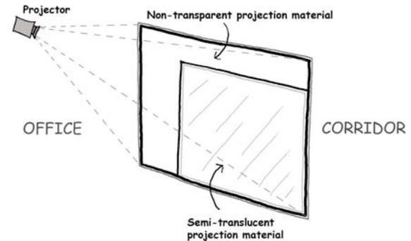
Figure 3. FrostWall projection onto a combination of opaque and semi-transparent projection material
