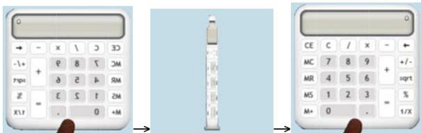
Figure 2. Graphically “flipping” interface elements on the FrostWall to face the user correctly
