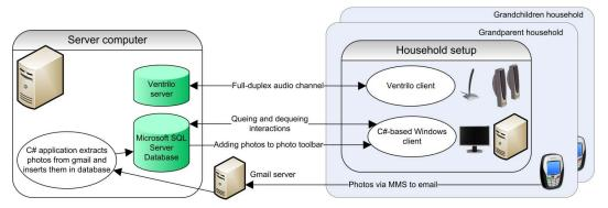
Figure 5: Technical structure of the system.
