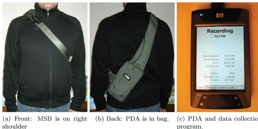
(a) Front: MSB is on right shoulder (b) Back: PDA is in bag. (c) PDA and data collection program.
