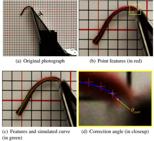
**Figure 11:** The experiment setup for bending tests (a). By using point features shown in (b), the optimization system finds a set of optimal parameters that matches the simulated mesh with the observed cloth shape (c). A correction angle  $\theta_{corr}$  shown in (d) is used as an intrinsic parameter to account for labeling errors.
