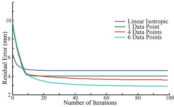
**Figure 9:** The convergence plot for modeling stretching behaviors, with data shown for Tango Red Jet Set. Using more data points, meaning more piecewise linear regions, helps the system converge to a lower minimum.
