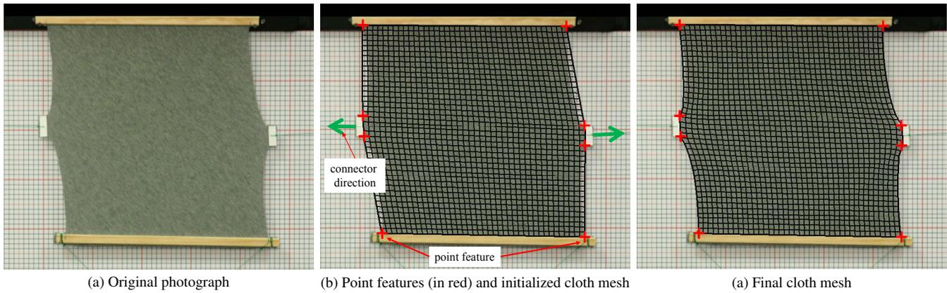
**Figure 8:** A 45° cloth sample shown in (a) is tested by hanging weights on its three edges. We use labeled point features (in red) to construct an initial cloth mesh in (b). Labeled connector directions (in green) are used as force directions in the simulator, so that the simulated cloth mesh finally matches with the observation as shown in (c). In (b) and (c) a grid of parameter lines from the simulated cloth has been superimposed on an image of the real cloth to allow comparison.
