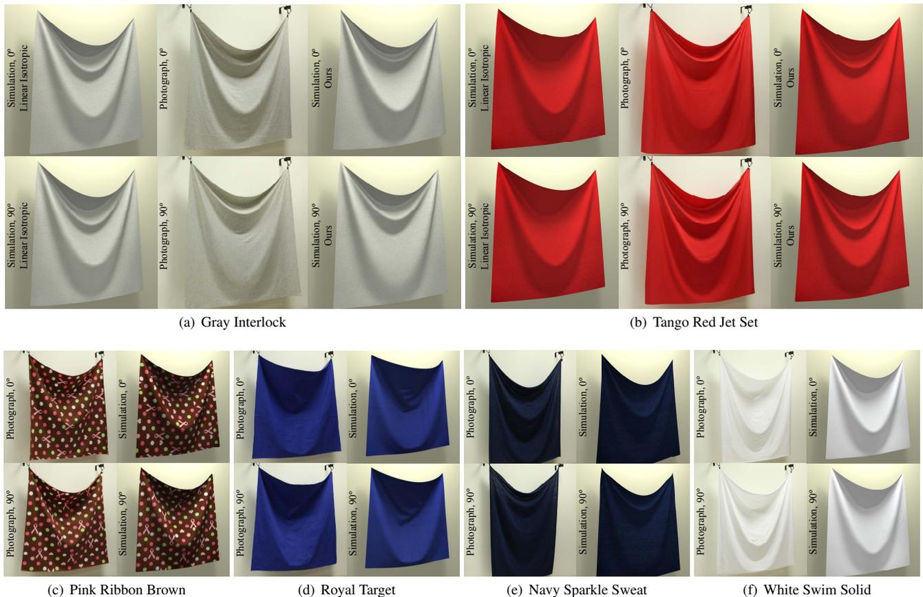
**Figure 14:** A comparison of real and simulated hanging sheets. By choosing various cloth materials, a  $1m \times 1m$  simulated cloth sheet is deformed into different shapes under gravity and compared to photographs of real sheets.
