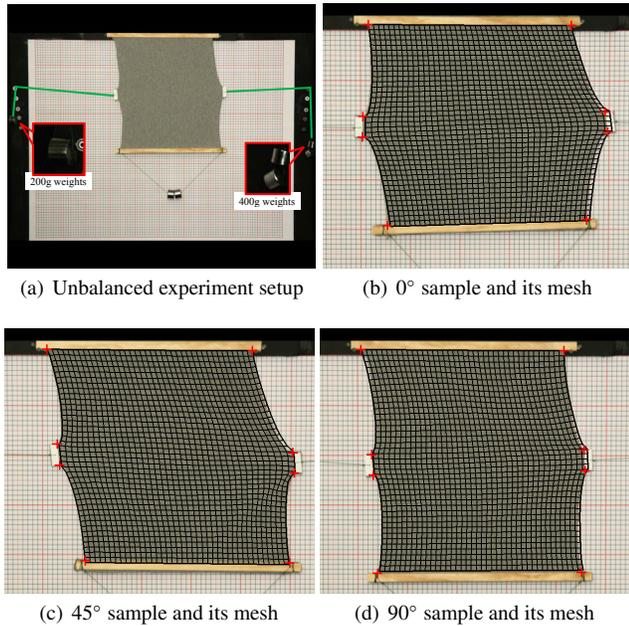
**Figure 12:** Unbalanced biaxial tensile tests for validation purposes. Simulated cloth meshes are rendered as a grid over the image to show the difference between their shapes and captured cloth sample shapes.
