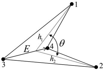
**Figure 5:** The bending angle and its neighboring triangles.
