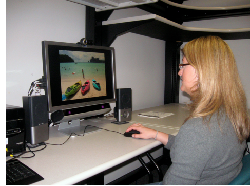
Figure 1: Photograph of experiment setup. The eye-tracking hardware is fixed to the bottom of the screen.
