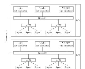
Fig. 19. Architecture of IDSS, running on two PCs.
