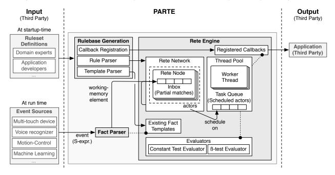
Figure 2: The architecture of PARTE
