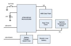
Figure 3. USB temperature logger schematic.
