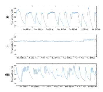
Figure 4. Logger data for three homes, all with set-points of 22°C, with (i) timed heating periods using an electronic proportional control thermostat, (ii) constant heating using an electronic proportional control thermostat, and (iii) timed heating using a mechanical thermostat.
