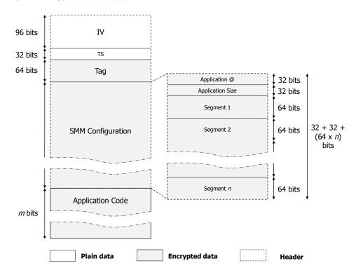
Fig. 7. Detailed flash application header, necessary to protect an application with the  $Load_{GCM}$  policy
