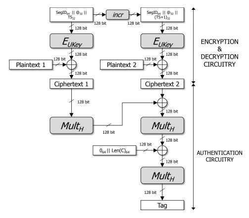
Fig. 5. The AES-GCM architecture for an authenticated encryption operation of a 256-bit plaintext cacheline.  $Mult_H$  denotes Galois field multiplications in  $GF(2^{128})$  by the hash key H, and incr denotes an increment function. The symbol || denotes concatenations between words. This figure was adapted from [National Institutes of Standards and Technology 2007].
