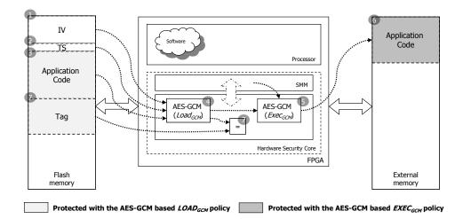
Fig. 6. Secure hardware architecture for application code loading. The SMM configuration is a part of the FPGA bitstream
