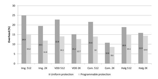
Fig. 9. Performance overhead of uniform and programmable protection versus no protection for four applications
