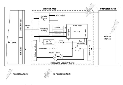
Fig. 4. Hardware security core architecture for a read request ACM Transactions on Embedded Computing Systems, Vol. V, No. N, September 2011.
