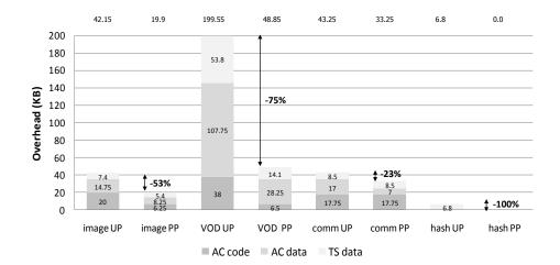
Fig. 10. On-chip security memory footprint for timestamp (TS) and authentication check (AC) tags for uniform protection (UP) and programmable protection (PP). The arrows indicate the percentage on-chip memory savings for programmable versus uniform protection
