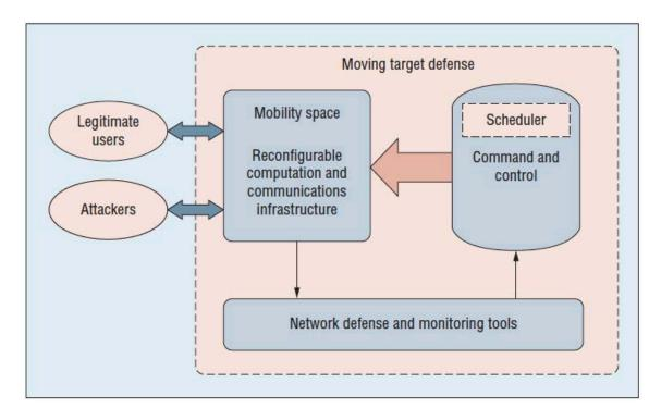
Feedback loop for a fully automated command and control
