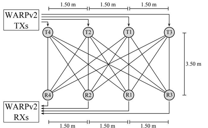
Figure 3: Experimental setup for measurements.
