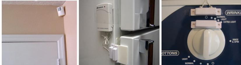
Figure 1. Sensor Use Examples: (from left to right) X10 motion sensor to detect users' entering a space (e.g., a room), or taking a book, X10 door sensor to detect users' opening the refrigerator, and X10 door sensor to detect the start or end of the laundry cycle.
