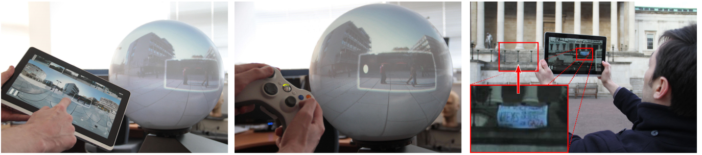
Figure 8: Additional displays and interactions. Left : Spherical display with a joypad controlling a cursor. Center : A tablet acting as a proxy controller, where the spherical display mirrors the context of the tablet. Right : Tablet display in situ, showing a protest that no longer exist in the real environment.
