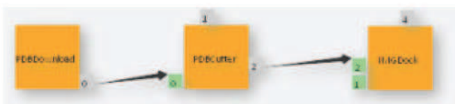
Figure 6: A gUSE workflow downloading a PDB file, splitting the stored complex into its receptor and ligand parts and performing a docking step.
