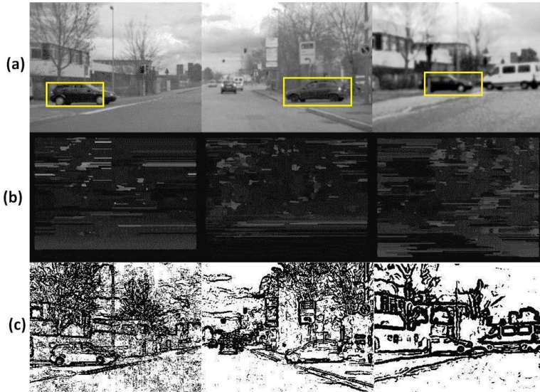
Fig. 10. Early simulation results for car side view detection on 320x240 images. A polynomial SVM of 50 reduced set vectors is used for classification. (a) Detection using depth and edge information (b) Disparity maps of input stereo images (c) Edge detection results for the input images
