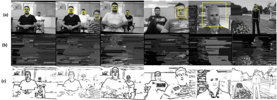
Fig. 9. (a) Detection using depth and edge information (b) Disparity maps of input stereo images (c) Edge detection results for the input images
