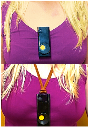
Figure 3 - Autographer clipped on (top) and with a neck strap (bottom). Yellow shutter is closed in both.
