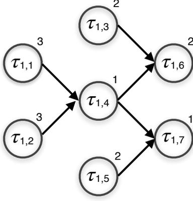
**Figure 1: An example of a DAG task  $\tau_1$  which consists of 7 subtasks. The number on the upper right corner of each subtask represents its WCET and the arrows represent their precedence constraints.**
