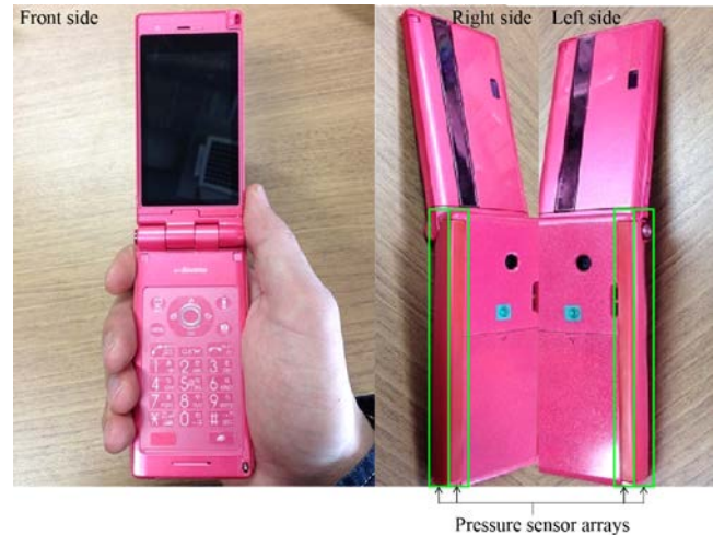
Figure 1. Experimental mobile phone with pressure sensors.
