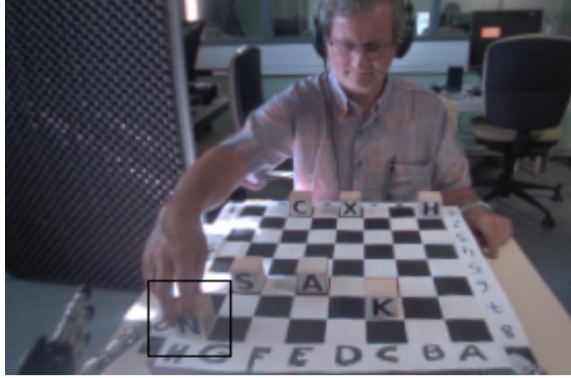
Figure 2: A sample of the pilot’s view on the chessboard via the right-eye robot (640x480 Dragonfly camera). The system instructs the manipulator facing the robot to a cube whose identifier (one letter) is only visible by the pilot via the robot’s eyes. The other faces of the cubes are left blank.
