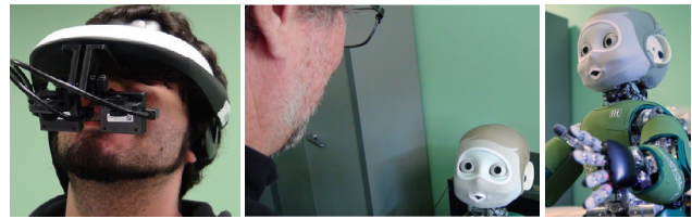
Figure 1. Our beaming platform consists of a HMD with an embedded Arrington® binocular eyetracker. The HMD receives input from Nina's eye cameras and ear microphones. Movements of the HMD are tracked by a Qualisys® motion capture (MoCap) system. The eyetracker and the MoCap system drive back Nina's head and eye movements.
