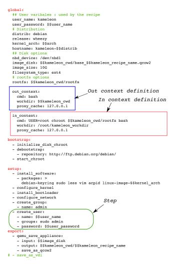
Figure 3: In the example, the section headers illustrate contexts (out\_context and in\_context), declarations (global) and sections (bootstrap, setup and export). This example uses a chroot jail as a container for building a software appliance based on Debian Wheezy.
