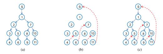
Figure 1. An example showing the directed graphs (a)  $T_1$ , (b)  $U_1$ , and (c)  $G_1$  for a network with n = 11 peers and m = 3. The node indices correspond to the peer labels for  $G_1$  and node S is the stream source.
