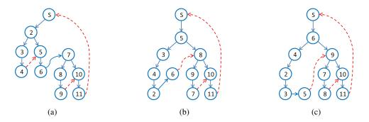
Figure 6. Topology of (a)  $G_1$ , (b)  $G_2$  and (c)  $G_3$  resulting from the departure of node 1 from Figure 2. Notice that the edges (3,6) in  $G_2$  and (4,5) in  $G_3$  have been broken to preserve the minimum length of 2 for the degree one chains.
