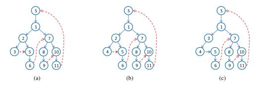
Figure 3. An example illustrating the change in the topology of  $G_1$ , from Figure 2(a), due to the departure of (a) node 4, a leaf node in  $T_1$ , (b) node 3, a degree one node in  $T_1$  and (c) node 2, a degree two node in  $T_1$ .
