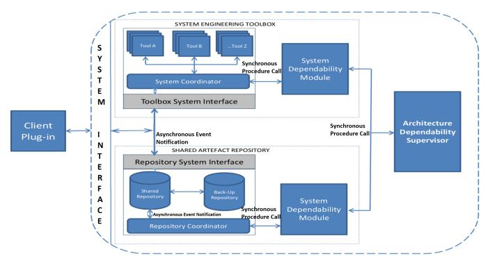
Figure 1: High-Level Representation of the Cloud-Based Architecture
