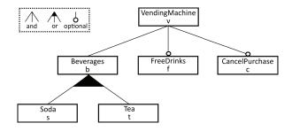
Figure 1: Feature diagram of vending machine SPL
