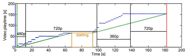
**Figure 1: Monitored parameters of an exemplary video streaming: current video playtime (green), buffered video playtime (blue), played out video quality/resolution (horizontal black lines). Events (vertical lines): page load (blue), playback start (green), quality switch (black), stalling (orange box), playback end (red).**
