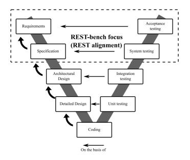
Figure 1: V-Model of software development
