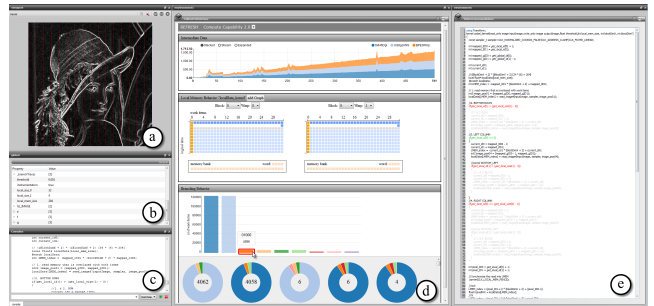
Figure 1: The interface of our integrated system: (a) shows a domain view that depicts the output of a Sobel filter and highlights corresponding to the hovered visual element, (b) shows a global variable view, (c) shows a console, (d) shows the visual explorer with different analysis views, (e) shows the source code editor with highlights that also correspond to the hovered visual element.
