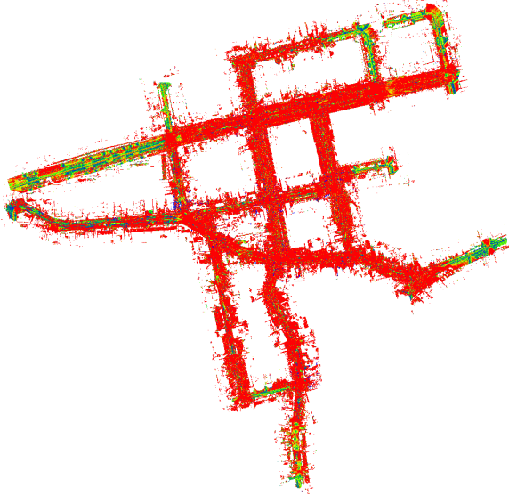
Figure 11. Latent map of the project area, before estimation (top view). Color scale: standard deviation, temperature scale, blue (0 mm) to red (7 mm or more).
