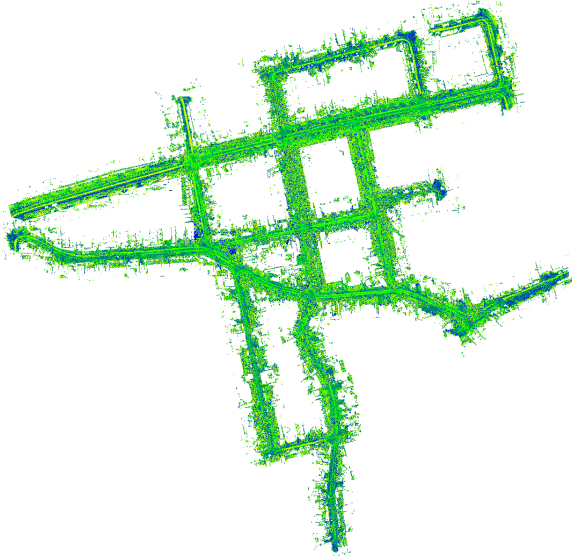
Figure 12. Latent map of the project area used in the last estimation (top view). Color scale: standard deviation, temperature scale, blue (0 mm) to red (7 mm or more).
