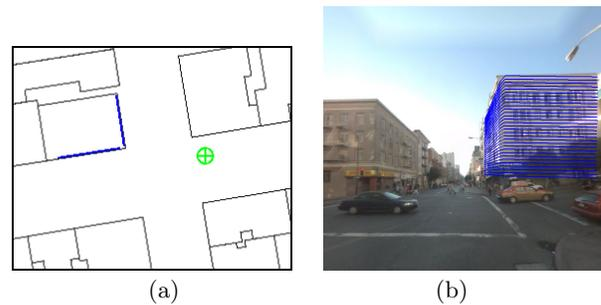
**Figure 2: Building height estimation.** (a) A map containing building footprints. The green marker represents the camera location. Blue edges indicate the part within the field of view. (b) A street level image. All blue lines are the projected edges with different elevation values.
