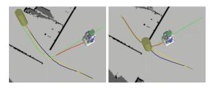
Figure 3: Robot stops not because of a planning failure but because it has planned a cooperative strategy where it waits until the human passes through.
