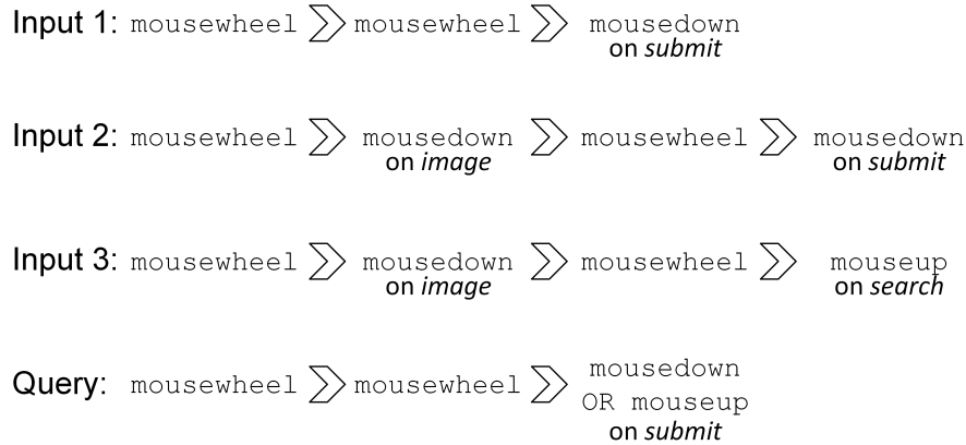
Fig. 4. How the query matches different inputs through Algorithm 1
