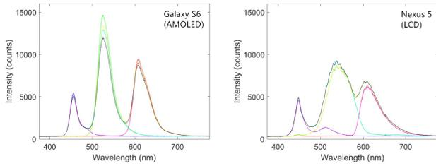
**Figure 5. Measured screen emission spectral for Galaxy S6 (AMOLED) and Nexus 5 (LCD). The line colors match with the screen colors (e.g., yellow line represents the yellow screen) except the black line which represents a white screen. These spectral show the wavelength range of the three color bands, which are activated in different proportions for different colors.**
